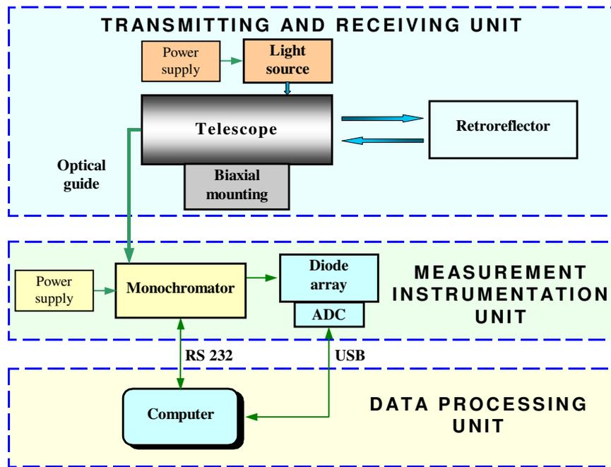
Fig. 2. The function chart of DOAS M1 spectrometers.
