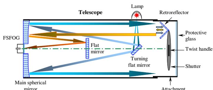
Fig. 4. Optical layout of the lamp signal measurement mode (top view).
