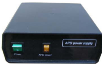
Fig. 9. Low voltage power supply of APD.
